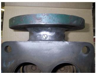
Into an old cracked valve with a broken flange, a pipe with a suitable diameter was inserted and fixed by using the PolymerMetal MM-metal SS-steel. Then this connection was secured by several screws.
