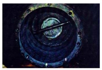
A worn out bearing bush of a floating dredger was rebuilt using MM-metal SS-steelceramic and Hardener yellow. Besides MM-metal SS-steel liquid type with Hardener yellow liquid was injected into a gap of 4 mm between bearing bush and boom.
